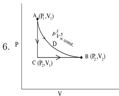
A gas is confined in a cylinder with a movable piston. It is observed that if the gas is adiabatically taken from state  $A(P_1, V_1)$  to a state  $B(P_2, V_2)$ , in the  $PV$  diagram it follows a path  $ADB$  whose equation is  $P^3V^5 = \text{const}$ .
